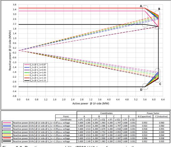
Figure 3-3: Reactive power capability (7500 kVA transformer variant).
