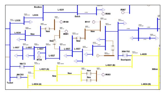
NSPI's records indicate that L-5027 radial section 9W-Tusket substation to 22W-Barrington Passage substation is 60.21km long. The line section from 21W-Lower Woods Harbour substation to 9W-Tusket is 50.41km in length, has wood pole H-frame construction with Linnet (336ACSR) conductor. The line has a 41MVA summer rating and a 60MVA winter rating. It is also restricted by relay rating at 39MVA and metering rating at 48MVA.
